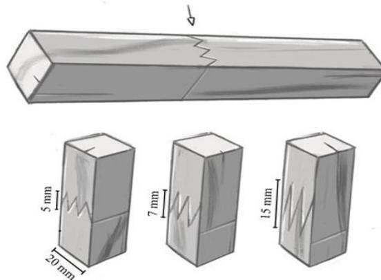
Figure 1 – Representation of the specimens (20 mm x 20 mm x 300 mm), with the three finger joint lengths used in this study (5 mm, 7 mm and 15 mm).
