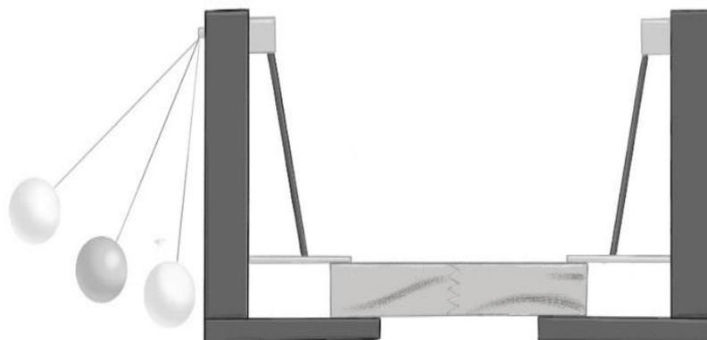
Figure 2 – Representation of the Metriguard Stress Wave Timer 239A equipment, applied to emit acoustic waves.
